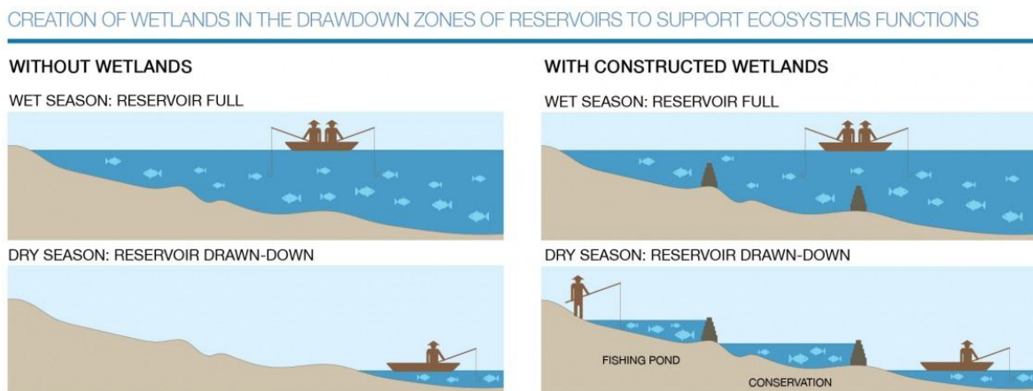
Figure 5.3: Schematic describing the operation of constructed wetlands within a reservoir (from Meynell and McCartney, 2014)
