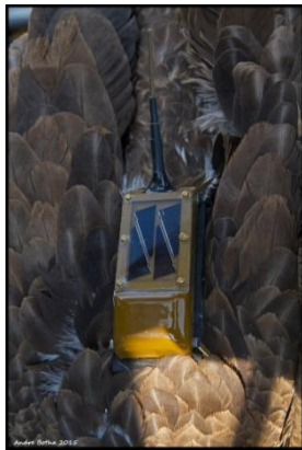
Figure 1. Satellite transmitter fitted on an African White-backed Vulture at Hlane, Swaziland.
