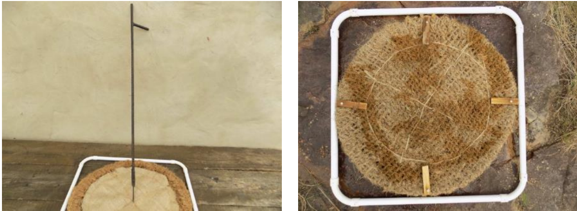
Figure 20. Left: Cold chisel with rebar extension and tap and twist handle; Right: completed net
