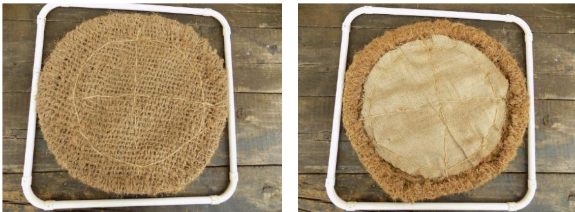
Figure 17. Left: Coir net outside view; Right: coir net with hessian inner lining
