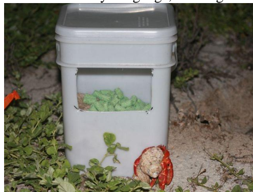
Fig 9.1 – rats can leap into these plastic stations but crabs struggle to get access.
