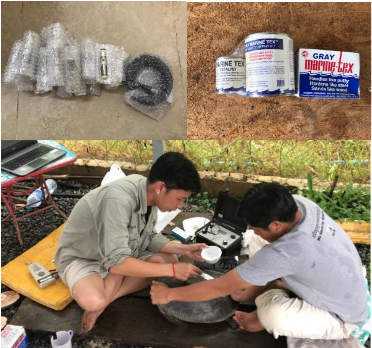
Figure 12. Transmitter and epoxy glue, and sticking a transmitter on a sub-adult terrapin
