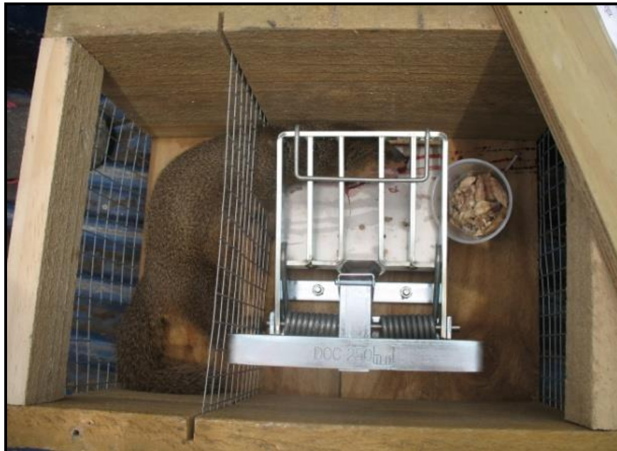
Figure 6. DOC-250 trap with the box lid rotated open to show the mongoose trapped in it at Satitoo. The wire mesh baffles that prevent the entry of other animals can be seen, with the bait still close to its original position. (Photo: Moeumu Uili)
