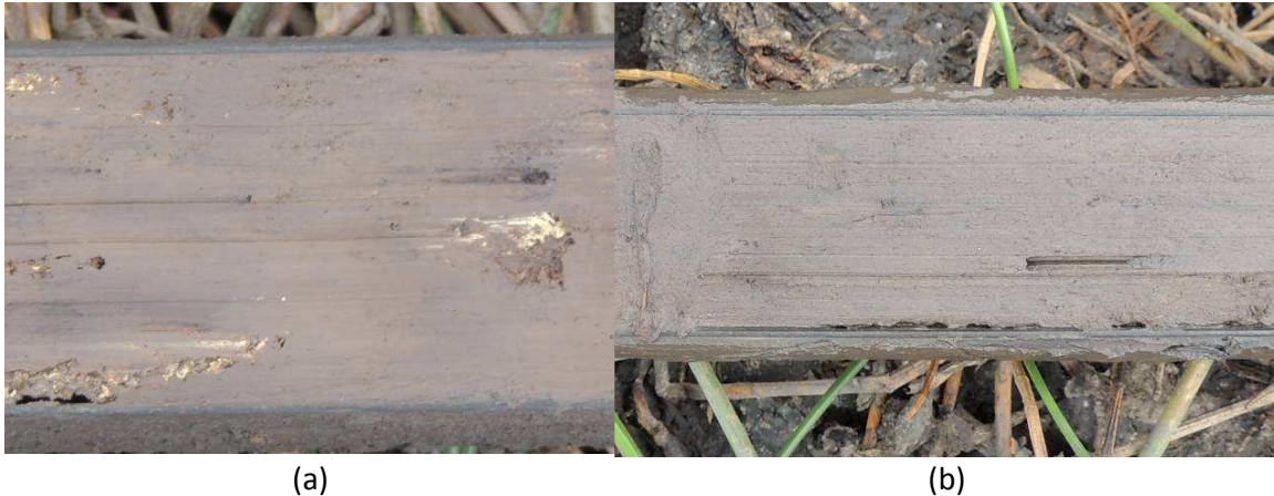
Figure 16. Features of acid sulphate soils: (a) A sulfuric horizon with jarosite minerals along root channels in acid sulphate soils, and (b) sulfidic horizon with pyrite minerals present beneath the sulfuric horizon or within 50-100 cm from the soil surface (Site 78).
