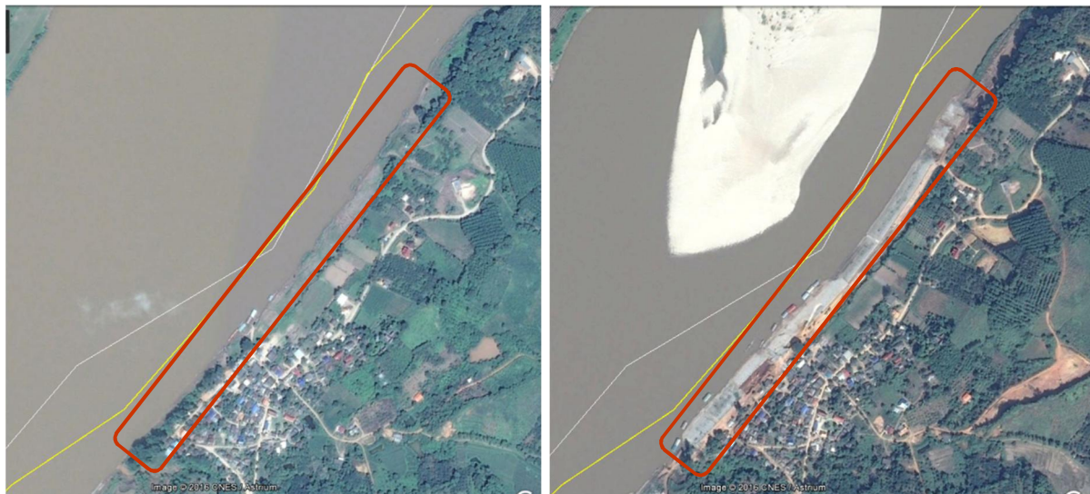
Figure 4.1: Construction of embankments between 2013 (left) and 2015 (right)
