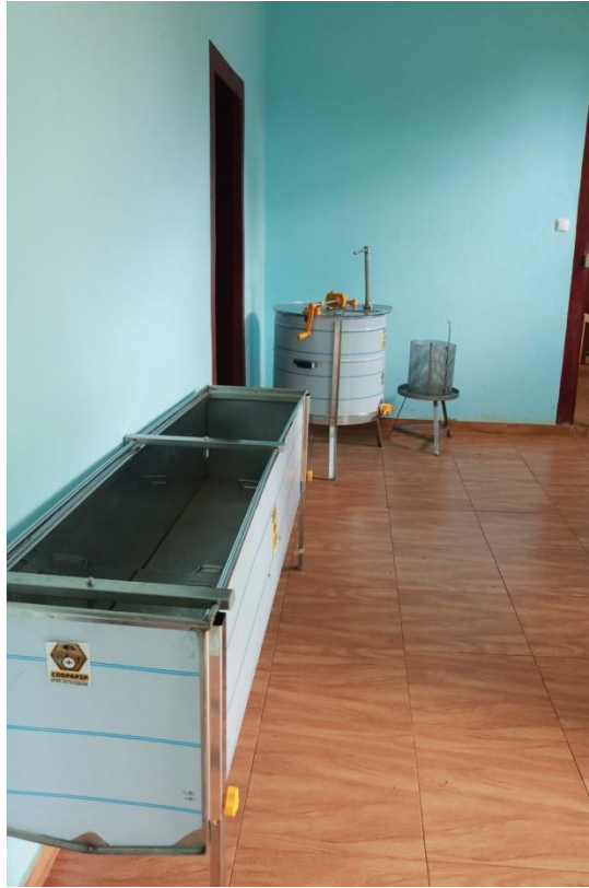
Figure 15. Honey processing equipment from the COOPAPIP honey house. From left to the right: uncapping table, centrifugal and manual press.
